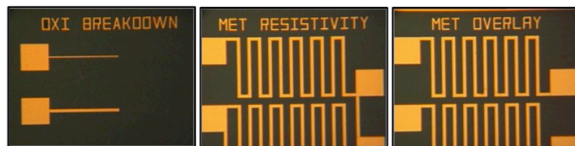
Figure 3-11: Illustrative pictures of first metallization layer lift-off.
